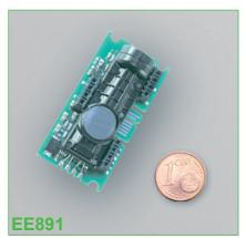
The CO<sub>2</sub> sensor EE891 has exceptional low power consumption! Because of the adjustable measurement interval, the average power consumption can be reduced to less than 60µA. The perfect solution for battery powered devices.
