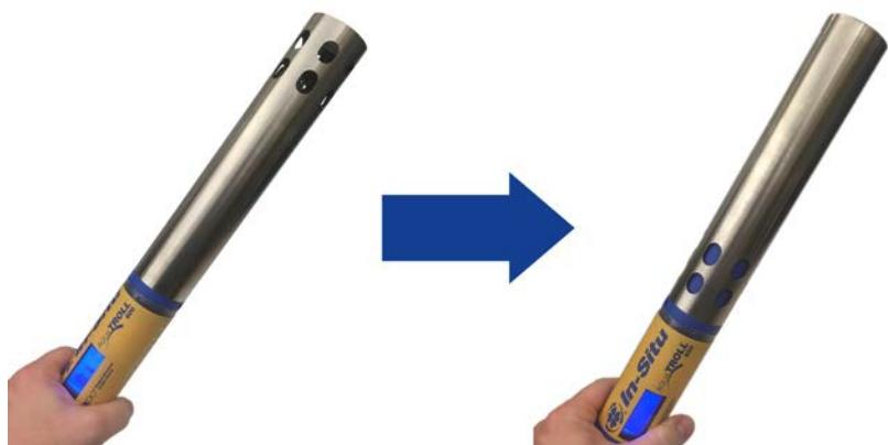
5. Invert the instrument so the sensors are facing up.
