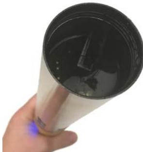
10. Move the solution in the calibration cell to ensure it has been in contact with the surface of the sensors and the inside of the calibration cell. If necessary, reinstall the blue top cap and gently shake.
