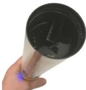
8. Move the solution in the calibration cell to ensure it has been in contact with the surface of the sensors and the inside of the calibration cell. If necessary, reinstall the blue top cap and gently shake.
