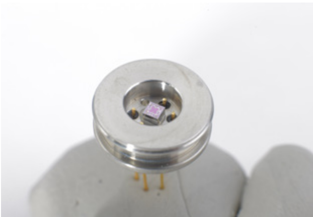
The silicon sensor element inside the glass-to-metal seal
